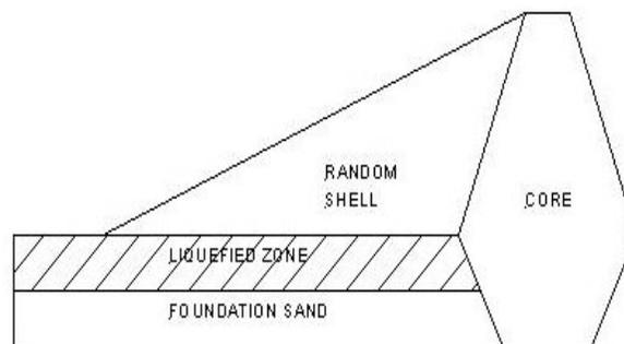
Figure 1a: Liquefied Zone Under Embankment Slope
