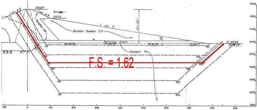
**Figure C-2a: Original Stability Analysis from “Embankment Criteria and Performance Report,” April, 1980.**
