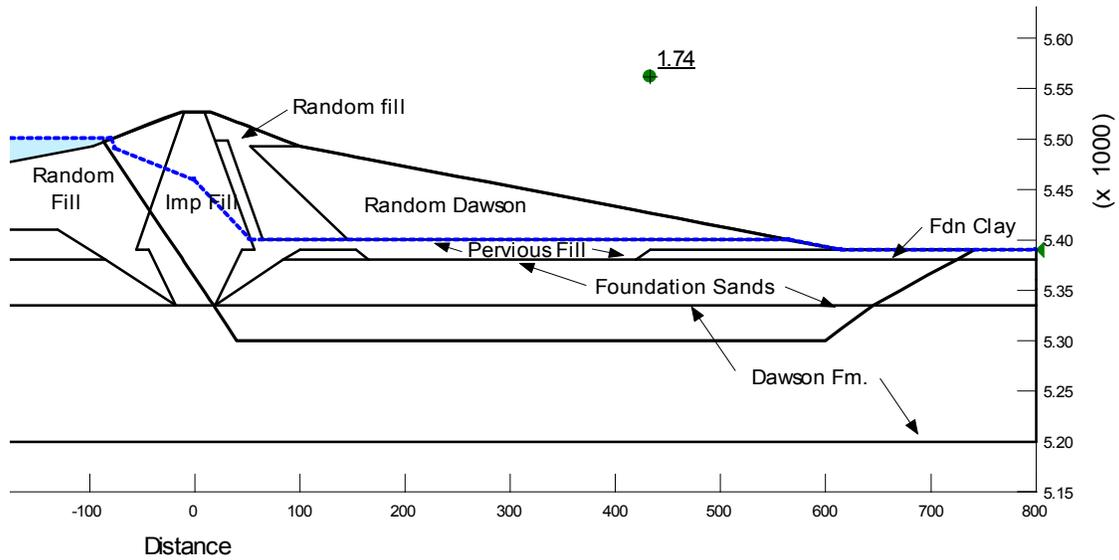
**Figure C-1b: Re-Analysis Output from Slope/W**
