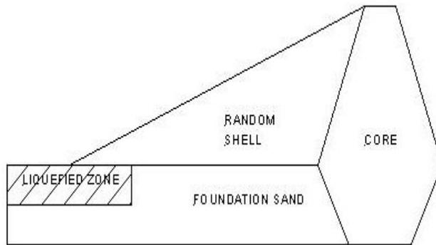
Figure 1b: Liquefied Zone Under Embankment Toe
