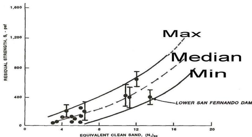
Figure 3: Relationship Between Residual Strength and SPT N-values (Marcuson, Hynes and Franklin, after Seed et.al.)
