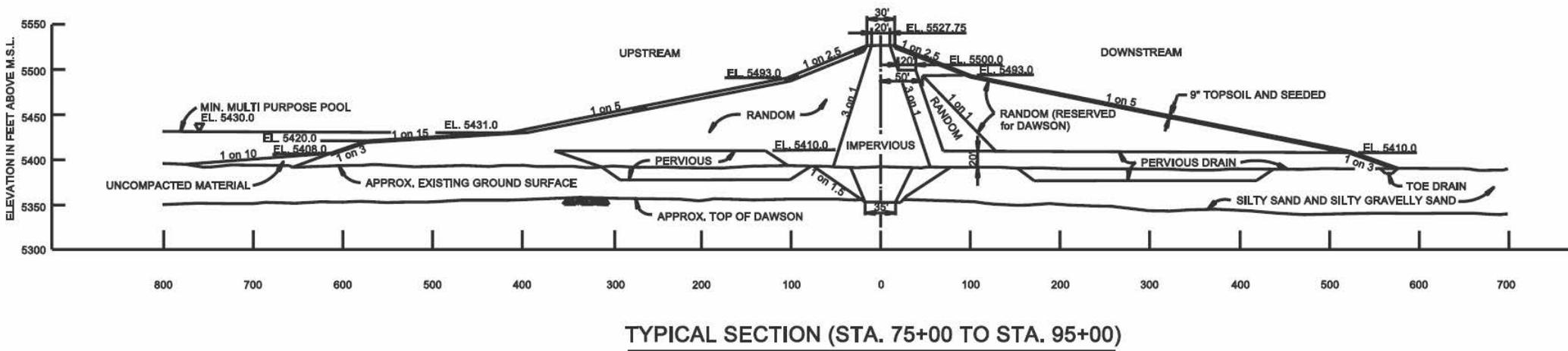
Figure 2: Embankment Zoning and Foundation Conditions in Valley
