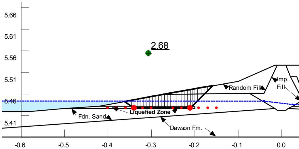
**Figure D-1: Post-Liquefaction Slope Stability at Upstream Toe**
