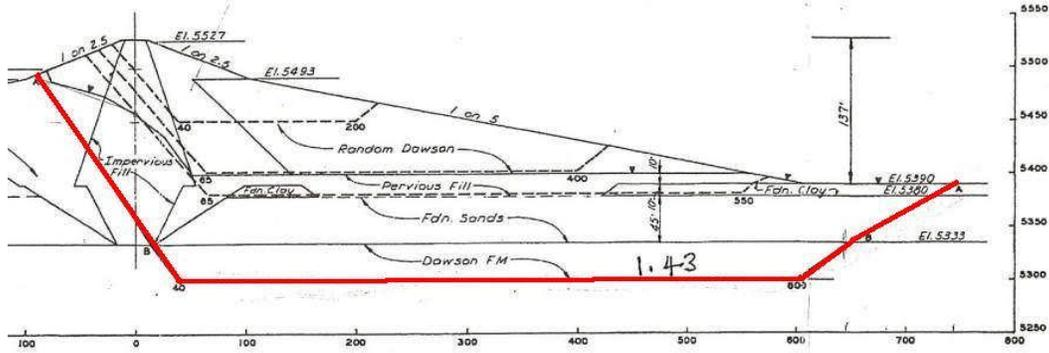
**Figure C-1a: Original Stability Analysis from “Embankment Criteria and Performance Report,” April, 1980.**
