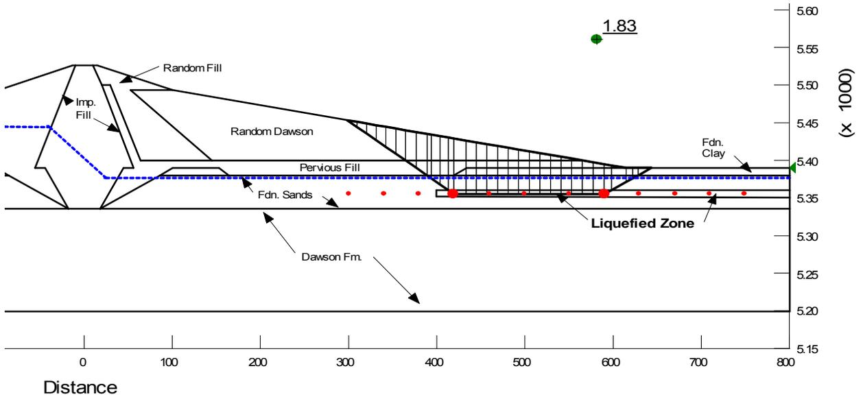
**Figure D-1: Post-Liquefaction Slope Stability at Downstream Toe**
