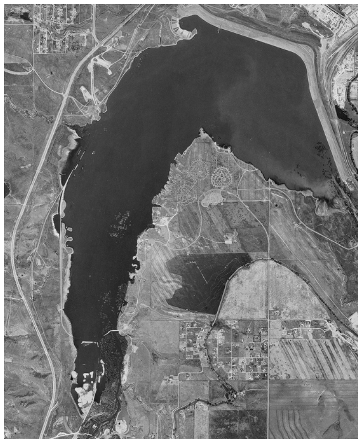
Aerial photograph from 1980 showing a flood at 5443' elevation. Notice that there were fewer facilities at this time, and some are inundated. Source: U.S. Army Corps of Engineers
